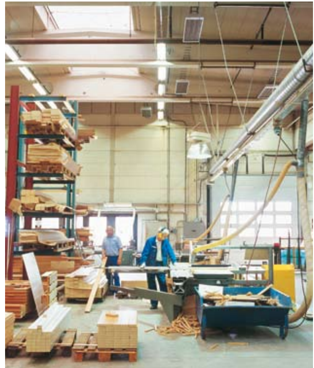
When using a conventional heating system, the warm air rises and stays under the ceiling and the cold air drops down to the floor. This is especially notable in buildings with high ceilings. Overheated air causes big energy losses. Radiant heaters on the contrary provide an even temperature.
