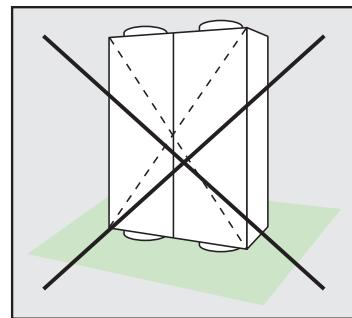
The unit can be suspended using threaded rods (M8) from the ceiling. The unit must be installed with a view to correct position of condensate exhaust. Other installation position is not possible.
